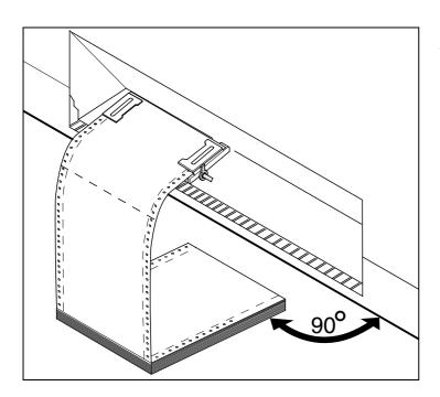
Make sure to align the paper stack in parallel with the printer and that the paper flow is unobstructed.
