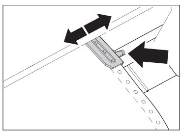
Open the coloured latch lever of the right-hand tractor and align it to the paper width.
