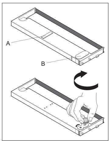
Remove the coloured protections **A** and **B**.
