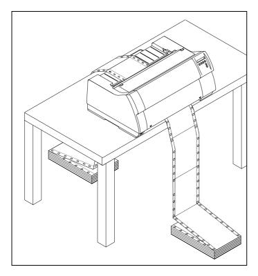
Place the printer on a solid, flat, surface, ensuring that the printer is positioned in such a way that it can not topple, and that there is easy access to the control panel and paper input devices. Also ensure that there is sufficient space for the printed output.
