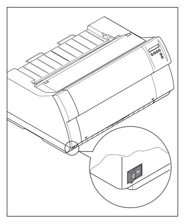
The power switch for switching on the printer is located at the bottom left at the front of the printer when viewed from the front.
