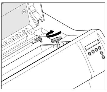
Insert the coloured tension knob into one of the two locations.
