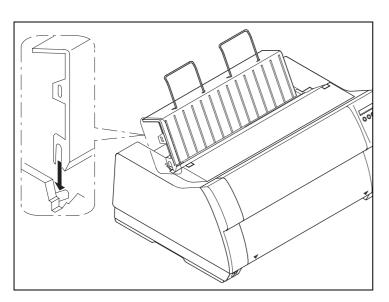
Make sure to align the paper stack in parallel with the printer and that the paper flow is unobstructed.
