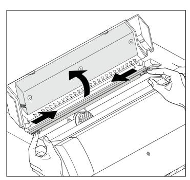
Move the coloured friction tabs to the left and right (direction of the arrows) as shown in the figure and raise the friction mechanism.
