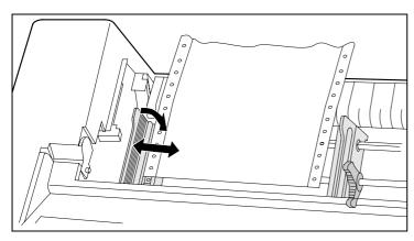
Release the coloured latch lever of the lefthand tractor and align the tractor in such a way that the first printing position on the paper matches the **X** mark on the printer housing.
