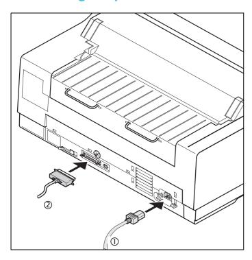
Connect the power cable ① to the power inlet of the printer. Connect the power cable plug to a mains socket.
