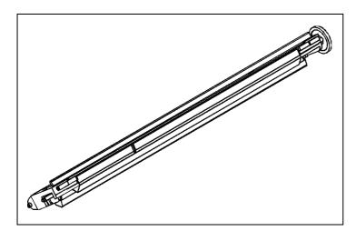
Clean the rollers of the upper friction as necessary with a mild cleaning agent and a soft, lint-free cloth.
