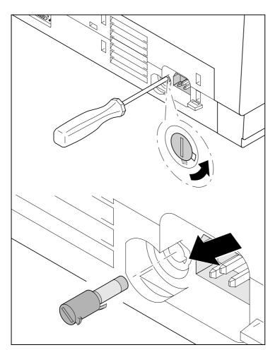
The printer is provided with a line fuse accessible from the exterior. Press the fuse cover slightly inwards with a screwdriver and turn it until the cover tab comes out through the recess in housing. Then remove the fuse.
