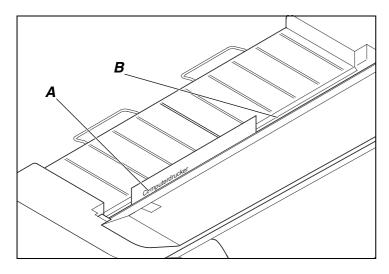
The paper is fed to the position where the bottom edge of the first printing line  $\bf A$  is aligned with the tear edge  $\bf B$  of the printer. The factory setting for the first printing position (TOF) is 12/72" (4,23 mm/1/6 inch). This is equivalent to the second line from the top.
