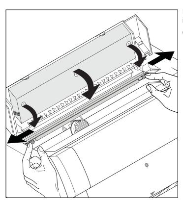
Press the friction mechanism down until it clicks into place.
