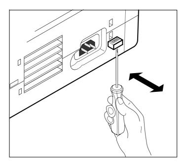
If the setting is incorrect, set the coloured switch at the rear of the printer to the correct position, using a pointed object (e.g. screwdriver, ball pen or tweezers).
