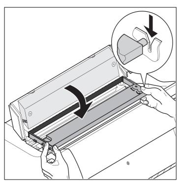
Slightly tilt the ribbon cassette forwards and thread in the ribbon between the coloured insertion tongue and the ribbon support (transparent plastic plate).
