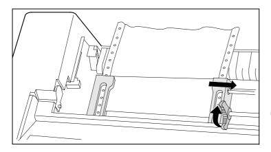
Release the coloured latch lever of the righthand tractor and align it to the paper width. Insert the fanfold paper into the right-hand tractor. Make sure that the paper form is inserted straight in order to avoid any paper jam. Close the tractor flap and lock the tractor by turning the lever towards the rear.
